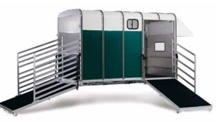
The containers have side-by-side stalls suitable for carrying horses of up to 16hh. They are constructed to the same standards as our horsebox trailers, with additional storage space in the Luton cab.
